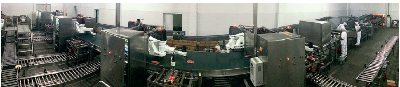
For the packaging of pickled vegetables, the Fu Ling Zha Cai company has opted for a pioneering line with multiple TP80 Fast Picker robots.
