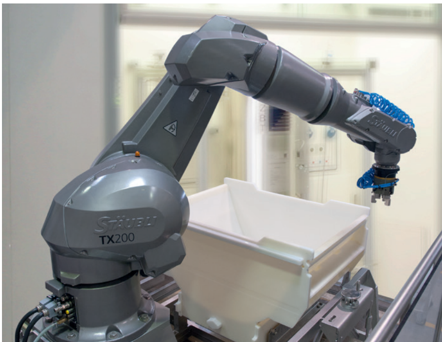
TX200 HE without the need of special protective covering, is used where handling tasks must be achieved flexibly and in tight spaces
