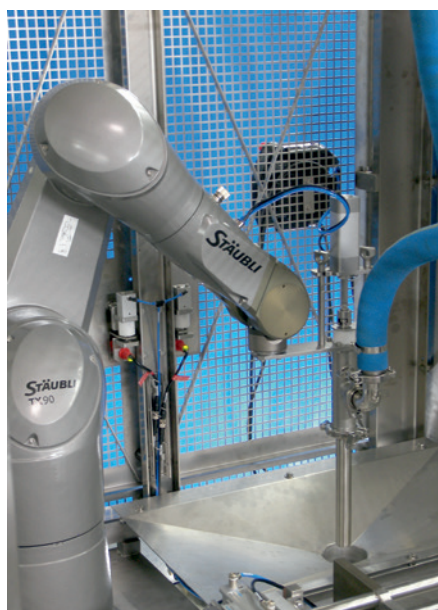
The Stäubli TX90 HE is at the heart of the filling line. These special robots can even withstand aggressive cleaning procedures.
