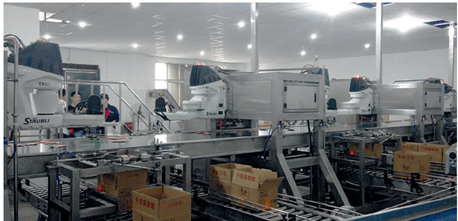
An image processing system determines the respective location and position of the sealed pots of pickles and relays the coordinates to the Stäubli robot controller.
