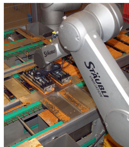
The enclosed Stäubli TX90L HE robot copes well with this crumbly product and the subsequent cleaning cycles.
